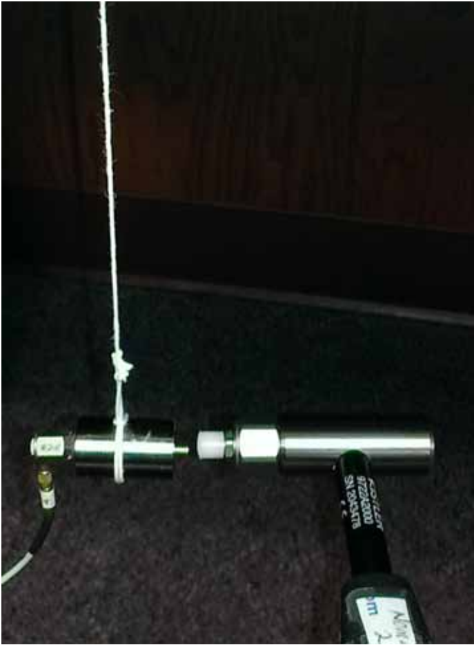
Figure 2: Improvised system to calibrate an impact hammer
