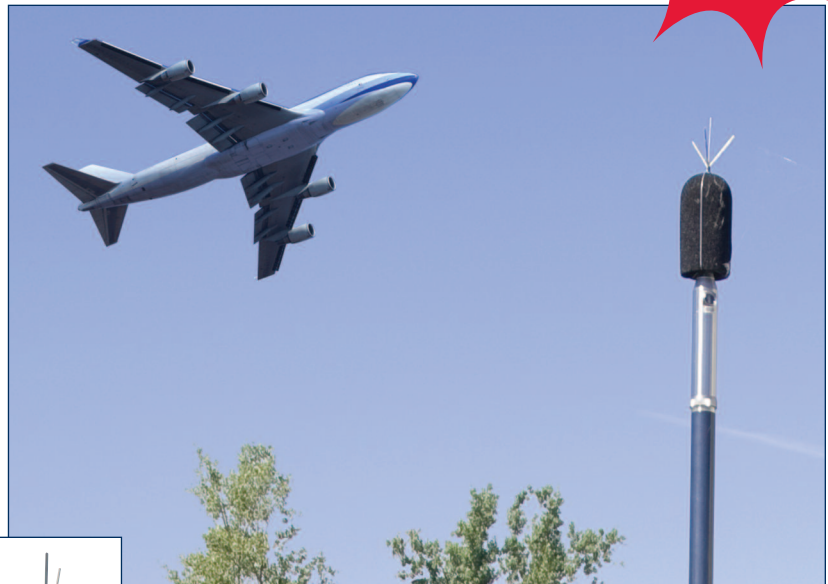
Typical Model 426A12-FF airport noise monitoring installation.
